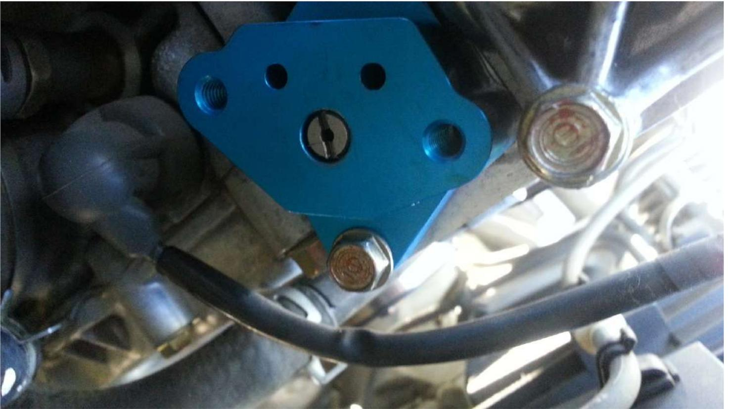
5. Install the oil plate on top of the now installed banjo bolt.
